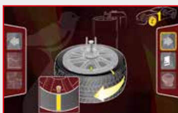
Match-Mounting procedure (rim-tyre)
